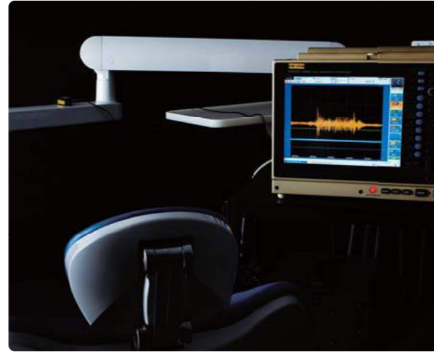
To achieve stable movement of the chair, an accelerometer is used to closely check warping of the unit during operation.
